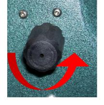
To increase the solution pressure, turn the regulator knob clockwise.
